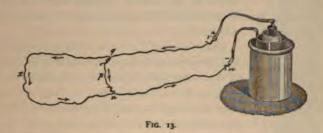
second wire, n, x, g be interposed, the current will divide at g, n, part going by way of g and part around through x, n. The divided currents which go through the wires are called derived or partial currents. If, instead of one or two wires, a large number were interposed, the current would subdivide itself as many times as there were wires, part going through each wire.
